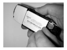
Lift the battery out by lifting from the bottom of the battery compartment.
