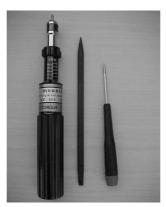
Shown left to right: Torque-limiting screwdriver (torque set at 28N-cm), fiberglass soldering aid, and T6 Torx+ driver.
