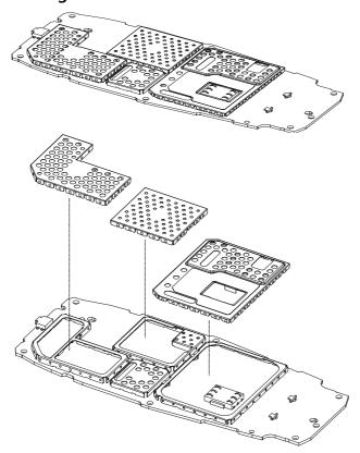
Remove shielding lids, as shown above. Do not re-use shielding lids once removed.
