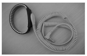
Some form of ESD protection should be used when handling the PWB and other electronic components. The photo above shows a wrist strap, which can be grounded to a bench. This or some other form of ESD protection should be used when handling the phone.
