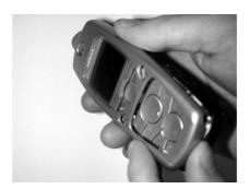
Place thumb under the edge of the A-cover and fingers on top. Pull the A-cover gently until a snaps deactivates.
